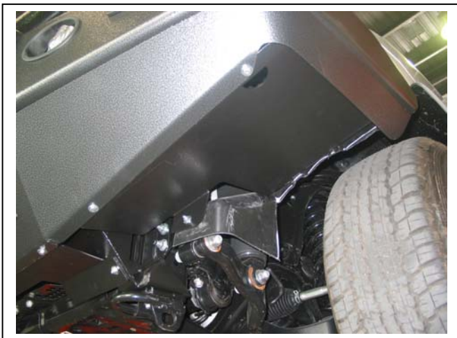
Figure 15: Passengers side under body guard.
