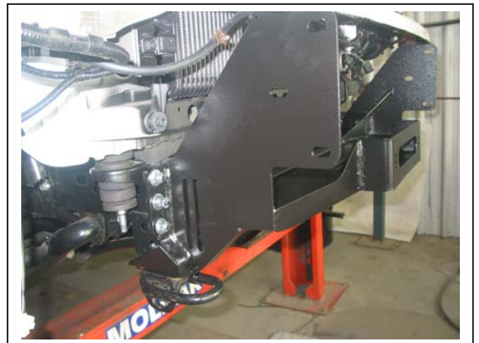
Figure 4: Three bolts to crash can assembly
