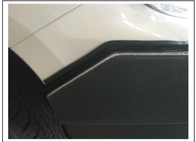
Figure 8: 3mm clip lock, trimmed to suit rear of cut
