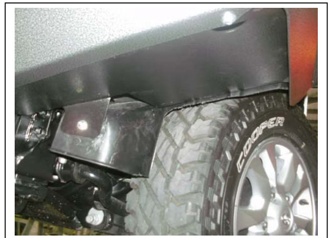
Figure 18: Inner guard, Passenger's side shown
