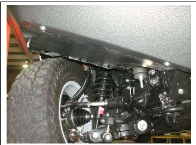
Figure 17: inner guard trim, driver's side shown
