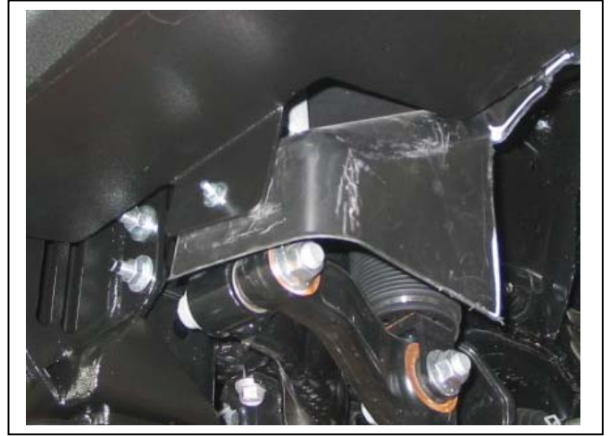
Figure 16: Front inner guard support. Passenger's side only
